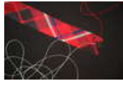
Conductive Thread inside a Fabric Bias Tube aka Tubes of Conductiveness by Lynne Bruning
